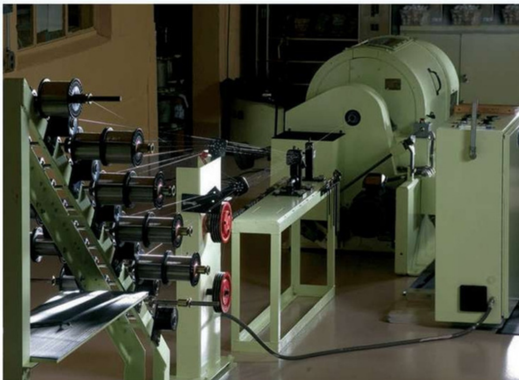
BUNCHER SET UP FOR STRANDING RESISTANCE WIRE
