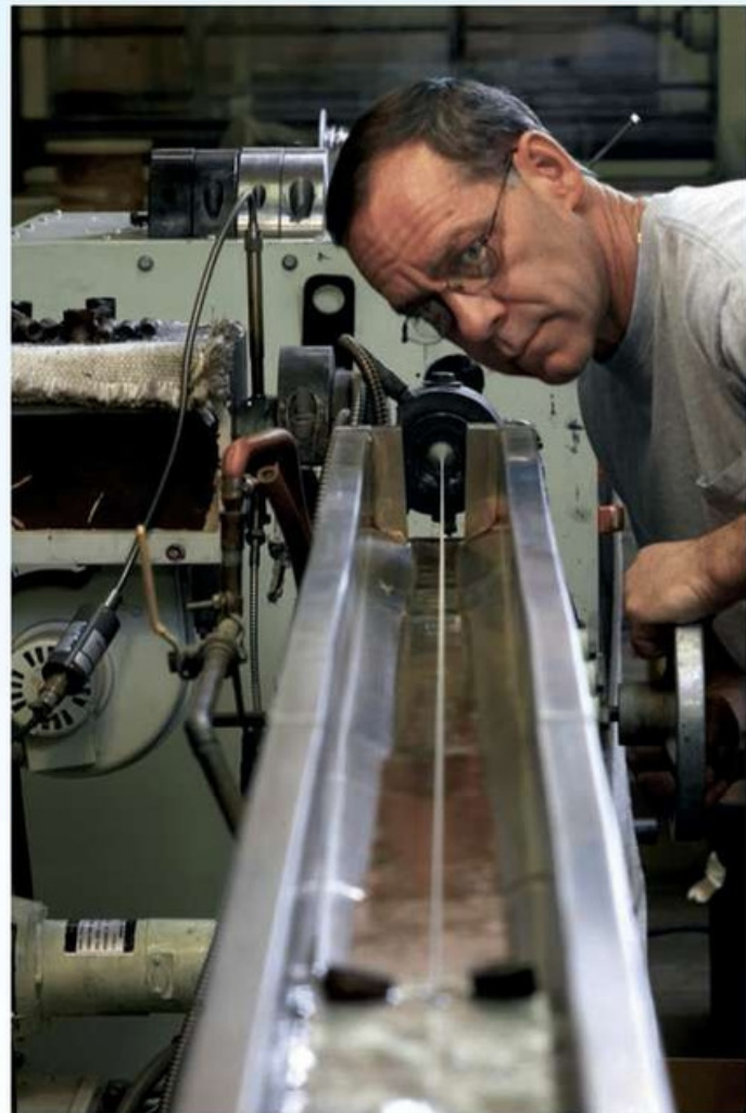
MELT EXTRUSION FOR INSULATING WITH FEP, PFA, AND ETFE
